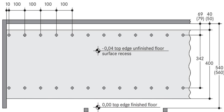
⊕ Measuring points at 100 cm points for checking the unevenness acc. to DIN 18202, table 3, line 2, or acc. diagram
