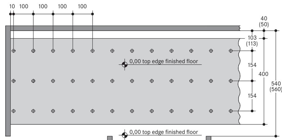
⊕ Measuring points at 100 cm points for checking the unevenness acc. to DIN 18202, table 3, line 3, or acc. diagram
