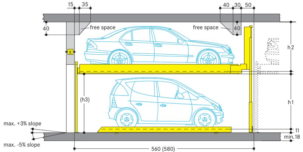
Width and height dimensions as well as further details for the building structure – see data sheet Combilift 551.
