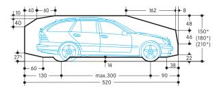
\* The total car height includes roof rail and antenna fixture and must not exceed the mentioned max. height dimension.
